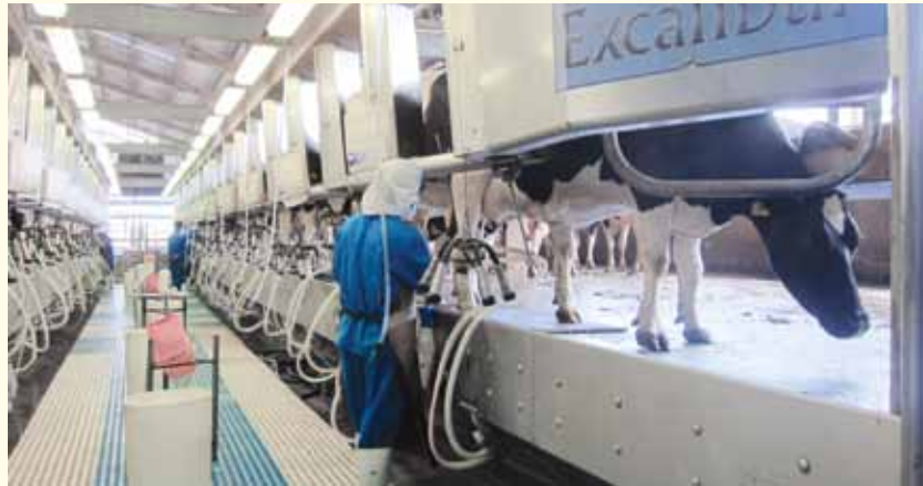
The cows at Greenfields are milked using Boumatic, a fully automated milking system where the milk goes directly from the cows to immediate chilling to 4°C via cooling stainless steel pipes with no human touch.
